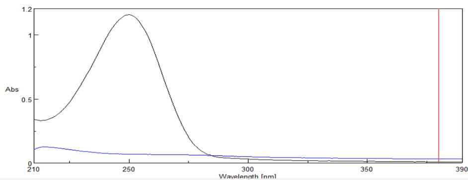
**Fig.1: UV Spectra of Glycyrrhetic acid at 254nm and Forskolin at 210nm**
